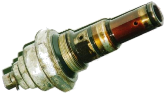
Figure 1: Sticky Servo valve coated in varnish (Courtesy of A. Sasaki)
