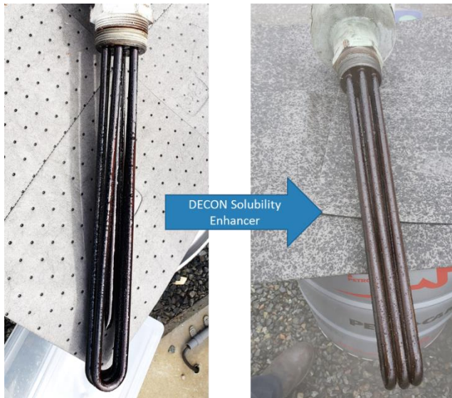
Figure 9: The impact of adding DECON, a solubility enhancing agent to an oil. One can observe the deposits have been dissolved. This was done while the equipment was operating, with no adverse performance benefits to the system
