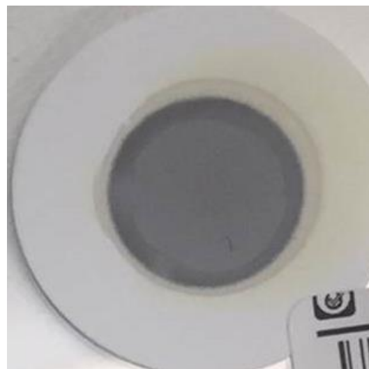
Figure 2: Silver MPC membrane from a mining excavator
